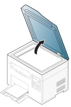
Place the original face down on the scanner glass. Align it with the registration guide at the top left corner of the glass.
